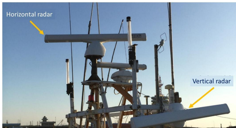
Figure 1.4.1-2 Radar Antenna Installed on the Vessel
